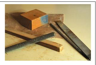
Step 5. The final fit. After a final sanding, the blocker may be left as is [seen full length (A) and close-up (B)], stained, or lightly painted. Make sure any final treatments will not be sticky and lead to a jammed door! Let this blocker rest in place without glue so it can be removed if needed (e.g., using a slightly shorter blocker to running a wire for Christmas lights). Barricade the gap throughout the year.
